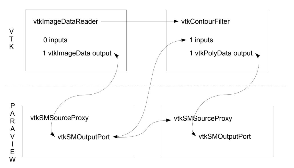
The ParaView client controls vtkAlgorithms that live on the server through vtlSMSourceProxies. For each output of an algorithm, ParaView adds a vtkSMOutputPort to the SourceProxy for the algorithm. ParaView uses SMOutputPorts to represent connections between algorithms, and can use them to update the pipline. For example, to gather meta-information.
