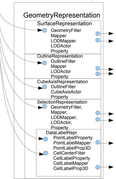
Representations contain Strategies. Strategies encapsulate the complexity of transporting data from the producing data server pipeline to the rendering pipeline(s). Depending on the data type and parallel configuration, the View will create different types of Strategy for any given Representation.
