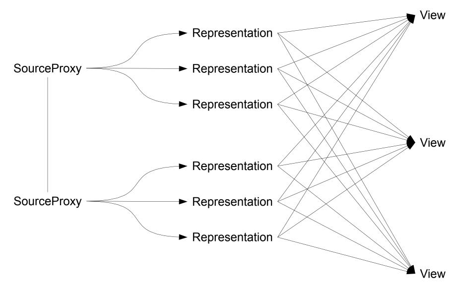
ParaView creates many rendering pipelines to show every SourceProxy in every View. The rendering pipeline is managed by a SMRepresentationProxy, which controls VTK objects such as Mappers, Actors and Properties. ViewProxies controls VTK objects such as Cameras, Renderers, and RenderWindows The exact type of Representation is a function of the View and the Data Type produced by the SourceProxy's i'th output.
