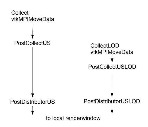
5 SimpleParallelStrategy – As configured for volume rendering of unstructured grid data in parallel configurations
