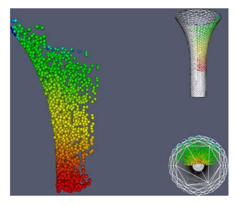
Figure 1: Results of the TestQuadraturePoints regression test. An unstructured grid with tetrahedral cells arranged in a cylinder is warped, clipped, and threshold-ed, before interpolating data fields to quadrature points and generating the quadrature point point set.
