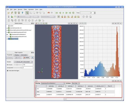
Figure 2: The new filters have been exposed in ParaView. This screen captures shows vector data interpolated to a fictional set of quadrature points, a table of basic statistics that has been computed on the interpolated fields, and a histogram generated using an interpolated data field.
