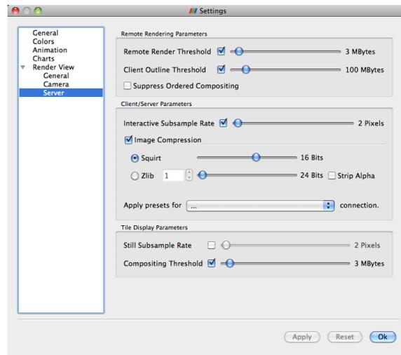
Like the other 3D rendering parameters, the parallel rendering parameters are located in the settings dialog box which is accessed in the menu from `Edit` → `Settings` (ParaView → `Preferences` on the Mac). The parallel rendering options in the dialog are in the `Render View` → `Server` section. The options have the following meanings.
