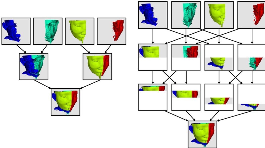
The wonderful thing about sort-last parallel rendering is that its efficiency is completely insensitive to the amount of data being rendered. This makes it a very scalable algorithm and well suited to large data. However, the parallel rendering overhead does increase linearly with the number of pixels in the image. Consequently, some of the rendering parameters deal with the image size.
