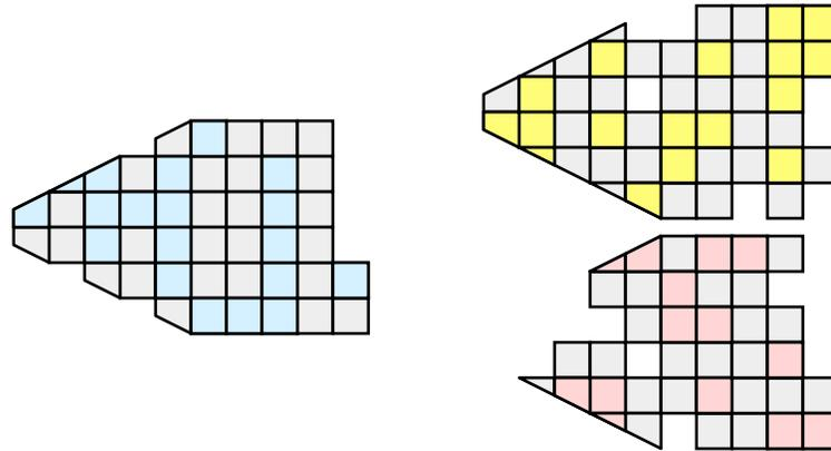
In this example, we see that a single level of ghost cells nearly replicates the entire data set on all processes. We have thus removed any advantage we had with parallel processing. Because ghost cells are used so frequently, random partitioning is not used in ParaView.
