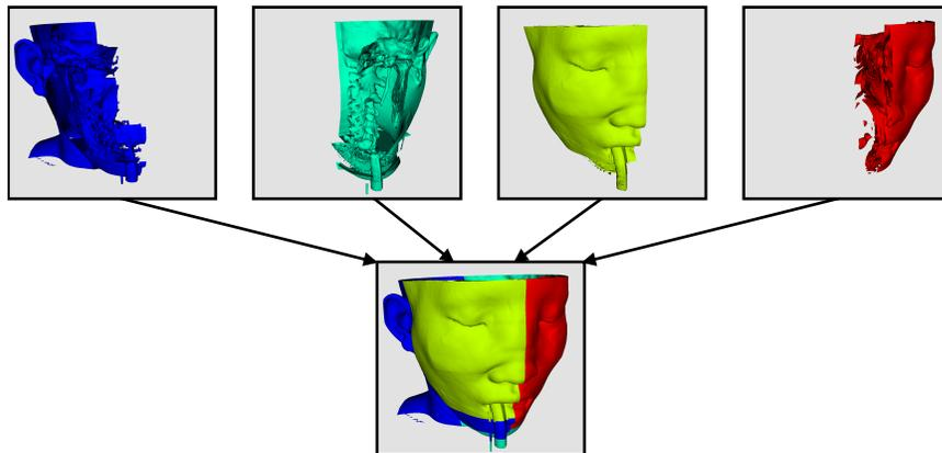
The preceding diagram is an oversimplification. IceT contains multiple parallel image compositing algorithms such as **binary tree** and **binary swap** that efficiently divide work amongst processes using multiple phases.
