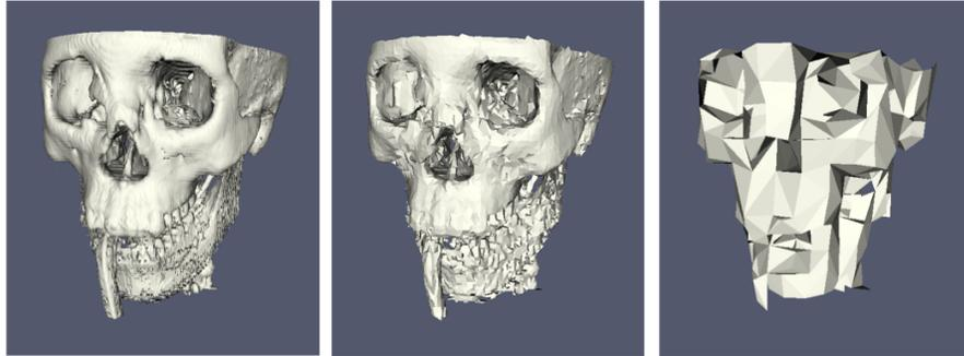
The resolution of the geometric approximation can be controlled. The decimation algorithm strives to place the polygons in a coarse grid. In the proceeding images, the left image is the full resolution; the middle image is decimation on a  $50^3$  grid, and the right image is decimation on a  $10^3$  grid.
