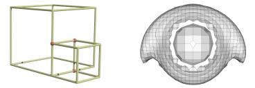
**Fig. 1.** Example of partly connected vertices (in red) and the corresponding cracks appearing after a contour algorithm is applied
