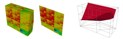
**Fig. 3.** Left: a 3D ternary tree-based AMR grid with 3x4x2 root cells, non-uniform geometry, and various levels of subdivisions, direction) planar cut thereof. Right: iso-contour across a 3D binary tree-based AMR grid overlaid over the edges of the wireframe representation of the dual mesh.
