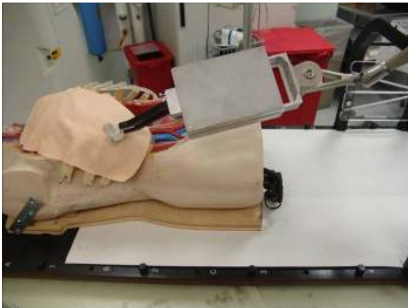
Figure 23.2: Robot assisted needle placement phantom study setup.
