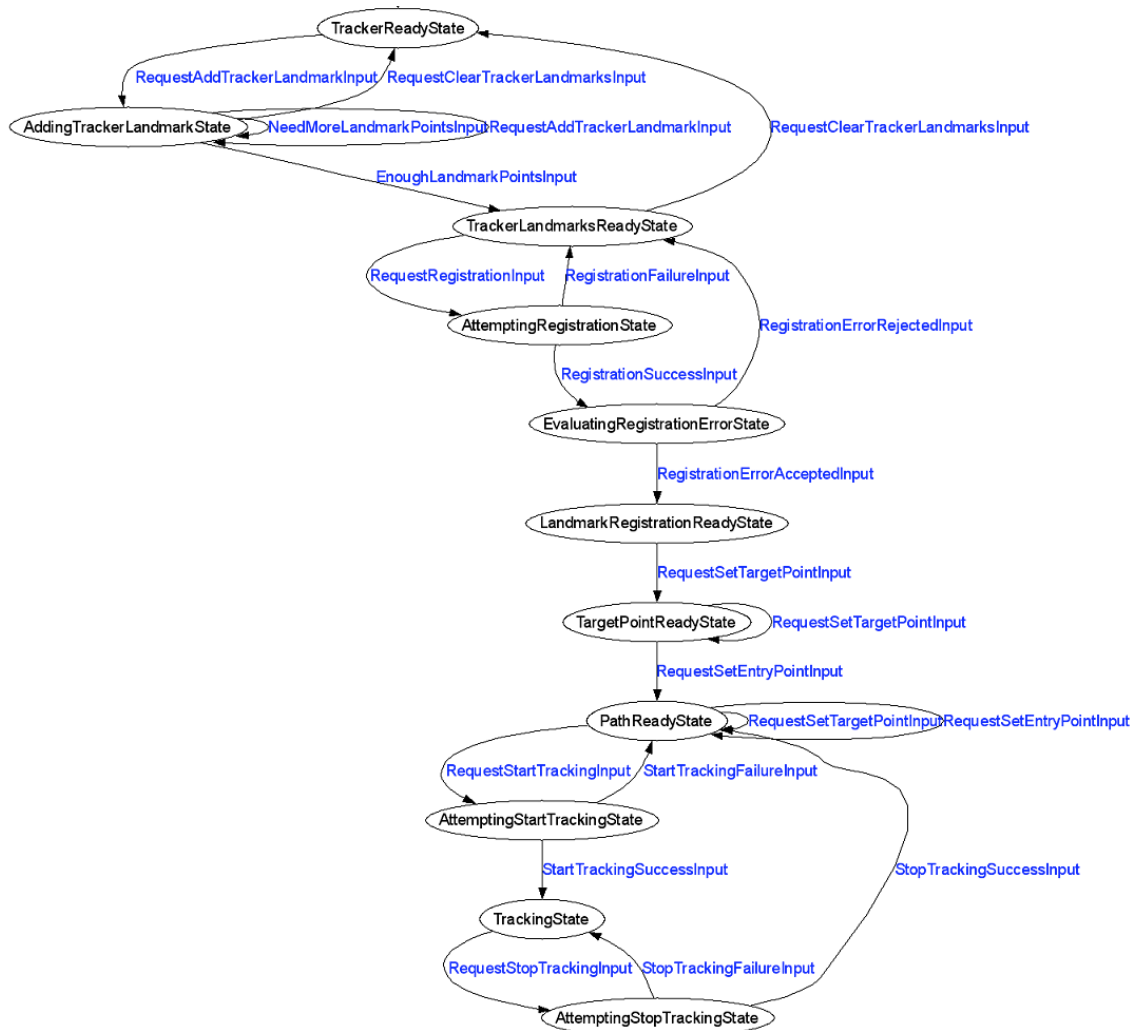
Figure 4: State machine diagram for example application (partial)
