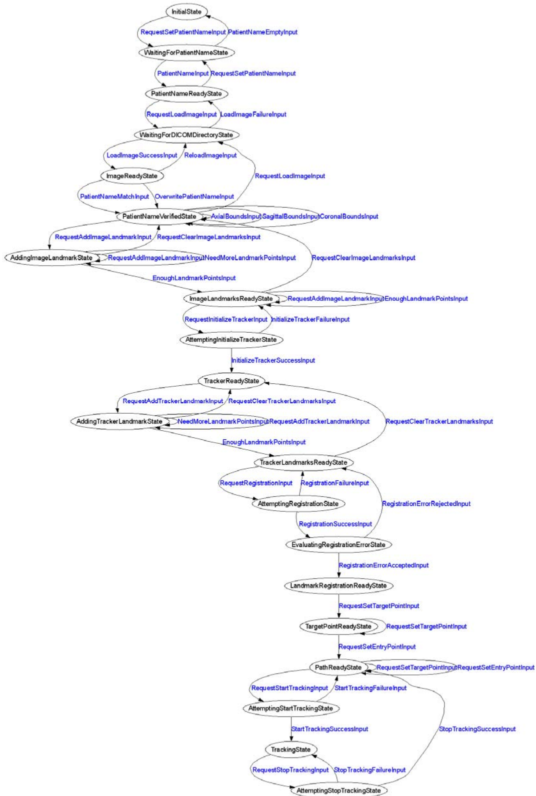
Figure 2: State machine diagram for needle biopsy application. (Circle for state and arrow for transition and corresponding input)
