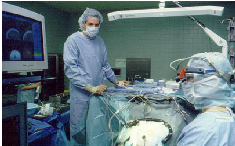
Figure 1. Image-guided system for brain surgery showing the optical tracking system at the top right and the display overlay on the far left. The patient is under the blue cover in the middle. (Photograph courtesy of Richard Bucholz, MD, St. Louis University).
